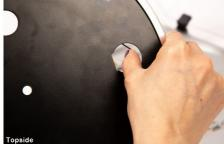
6. Gently lower the platter onto the central spindle of the base unit, ensuring that the elastic band is stretched over the drive shaft.
